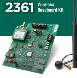
2361 Baseboard Kit plugs into the 1830 series controller main circuit board to provide the controller with a wireless wiegand connection.
