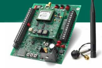
1489 Expansion Board Kit plugs into the 2358 circuit board (shown) to provide the Tracker Expansion Board with a wireless wiegand connection.
